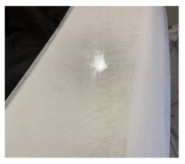
This issue can cheaply and easily be resolved by the application of thin rubber Heat shrink grip. This material is readily available from ebay and is available in various sized to suite the diameter of your tiller extension and in a range of colours. Simply slide the material over then extension and with a heat gun warm it and it will shrink tightly over for a permanent fit.
