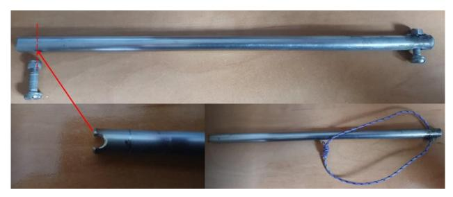
A more expensive but convenient method of attaching the Jib tack is the introduction of the Selden 50mm Quick release snap shackle adapter. This is simply bolted to the Tack bar spigot. This enables quick release of the jib tack and is available from most Chandlerys. It's important to ensure the bottom bolted section is protected so it does not catch on the kite.
